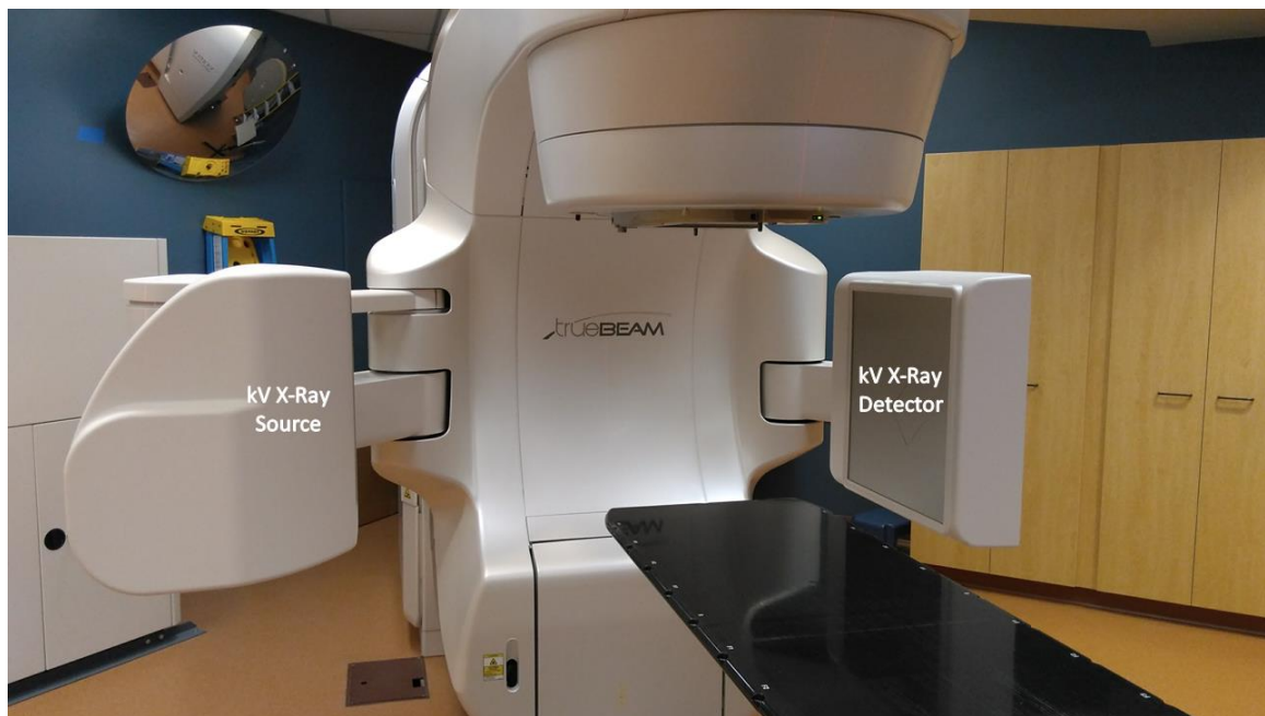
Figure 3: Linac OBI with kV x-ray source and detector labelled.
